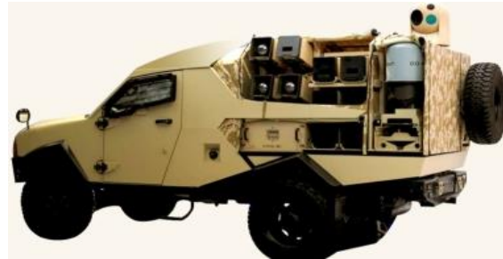
Figure 2. Spike NLOS B-vehicle mount
